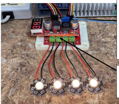
Using the adjustment screw on the blue multi-turn potentiometer adjust the output voltage to set your desired brightness. Excessive voltage may damage some lights, use caution when first powering on. Premium boards as shown have a digital display showing the voltage. LEDs typically use between 3.2 and 4.5 volts
