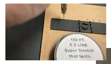
Drill out holes for truss rods if desired using the #62 drill bit also needed for the coupler screws.
