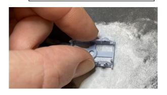
Sand the tops of the trucks smooth for proper operation.
