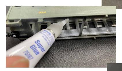
Use superglue or other clear setting tack adhesive to install window glazing.
